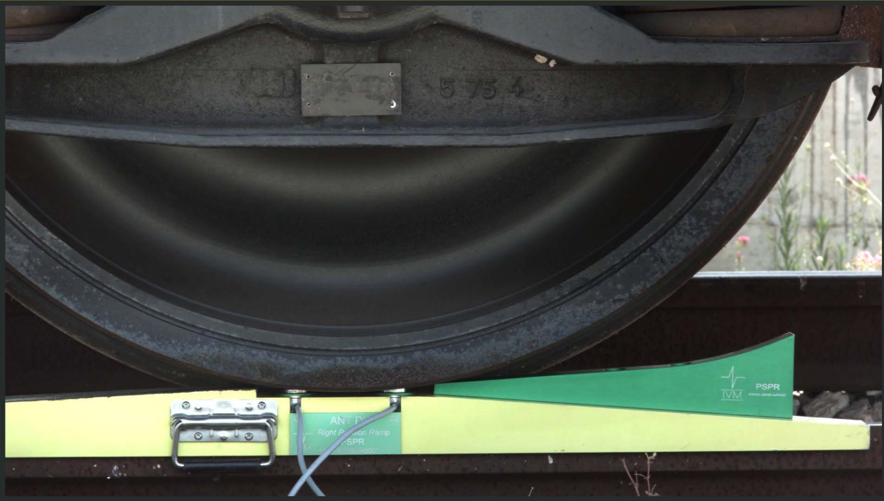
WHEEL CENTERING IN THE MEASURING ZONE
