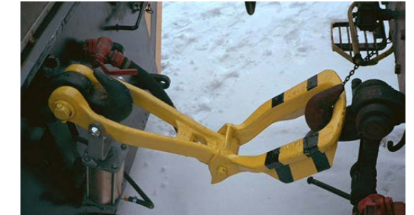
THE COUPLER IS LOOSE
